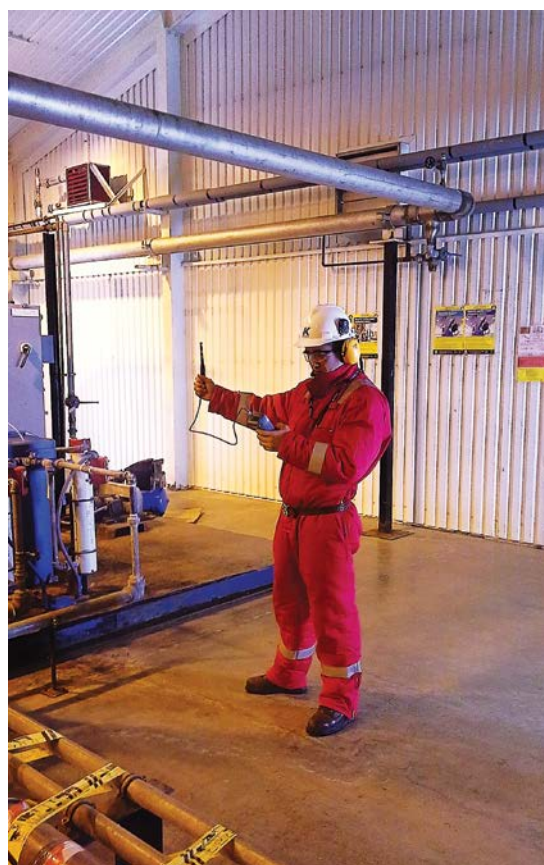
Measuring noise levels at an operating facility
