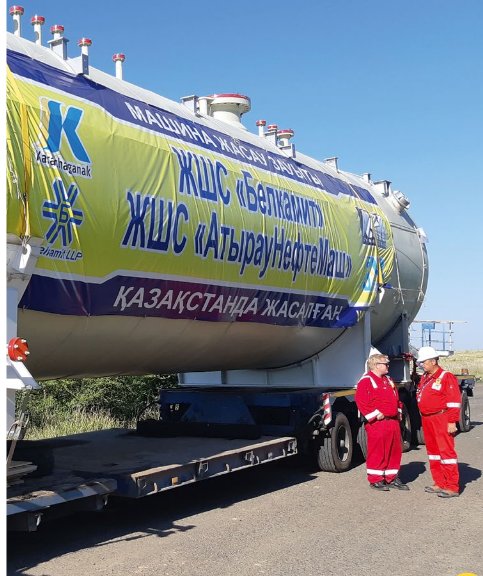
Super heavy thick-walled separator manufactured in Qazaqstan and supplied to the Karachaganak Processing Complex
